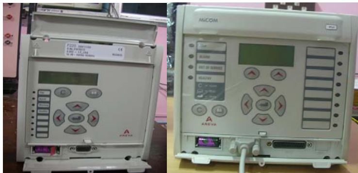
(b) Numerical Directional Feeder Management Relay of Type MiCOM P-141, Type no. P141311A1M0440J
